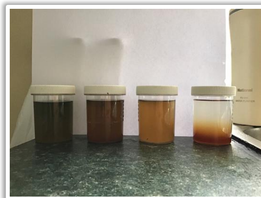
Water Testing Result – From Left to Right, Unfiltered, Nazava Filtered, Sawyer Filtered and Main Water Filter
